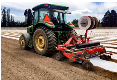
Figure 1. Equipment used for shaping beds and laying plastic mulch and drip tape.
